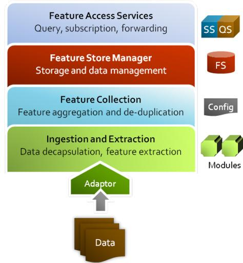
Figure 4: Illustration of the FCCE core modules, handling feature extraction, collection, storage, and access services.
